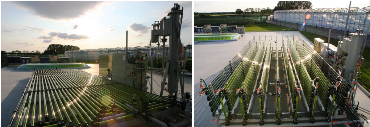
Figure 2: Tubular photobioreactors, horizontally (on the left) and vertically (on the right) stacked, at AlgaePARC (Wageningen, Netherlands).
