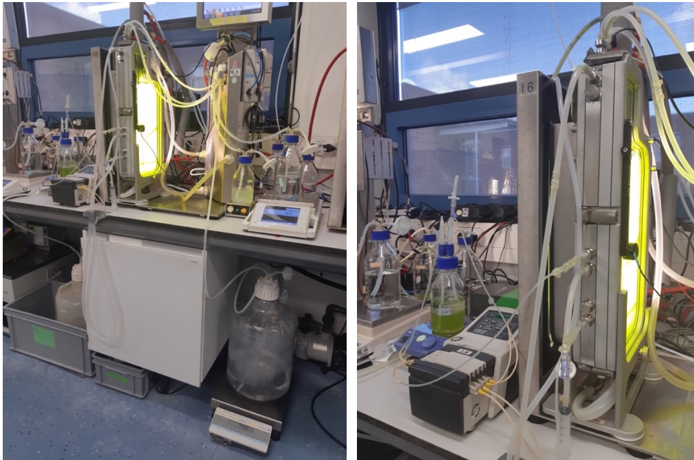
Figure 11: Set-up during the experiments with Infor reactors. Underneath the bench there is the overflow bottle on the left and the fresh medium vessel on the right, on the scale. On the right side of the reactor the antifoam and the base bottles can be seen, the latest on a scale. In front of the reactor there is the water lock. The extraction vessel and pump are on the left side of the reactor. To be noticed that the reactor surface would usually be covered, so that the only incident light was from the LEDs.
