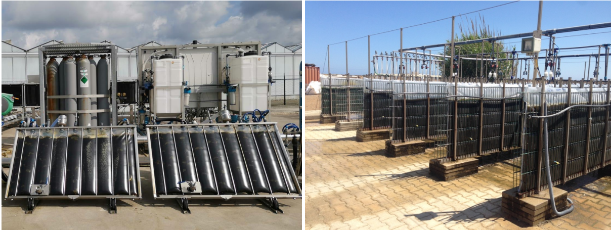
Figure 3: Flat panel photobioreactors at AlgaePARC (Wageningen, Netherlands) on the left, and at Necton (Olhão, Portugal) on the right.
